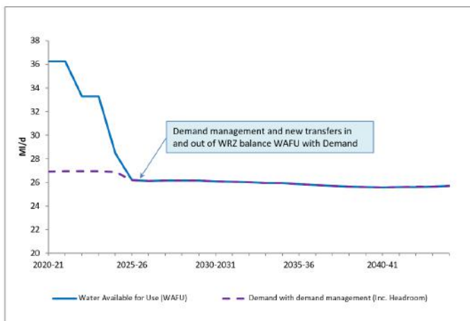
Figure 3.3.4: North Fenland WRZ final supply-demand balance to 2045 for dry year annual average (DYAA) conditions
