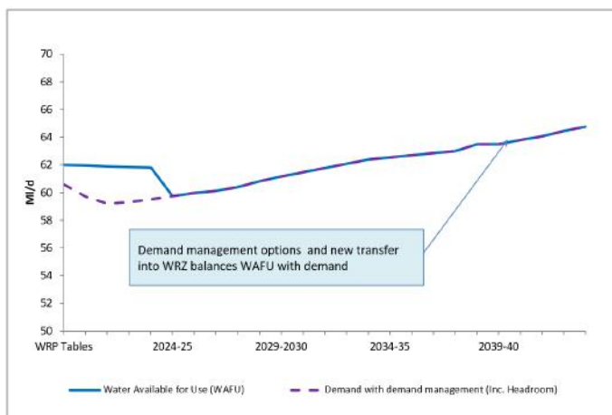
Figure 5.5.4: South Essex WRZ final supply-demand balance to 2045 for dry year annual average (DYAA) conditions
